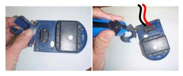
Next, you will need to remove the **small black rubber gasket** that keeps the place where the wires join the electrical contacts (below left). Be sure to keep this gasket clean and to replace it when you put everything back together. The screwdriver is pointing to the light blue contact box. There are two very small Phillips head screws that hold the wires in place. *These screws strip very easily, so make sure you have a small Phillips head screwdriver available to loosen and tighten them.*
